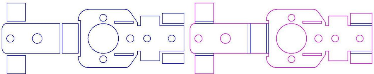
Now that we have a fully drawn object, it needs to be placed in the sheet for etching. This sheet is usually referred to as the fret. You may want to simply produce a lot of the components, as I would normally do, or you may want to incorporate it is a larger fret with other components.
