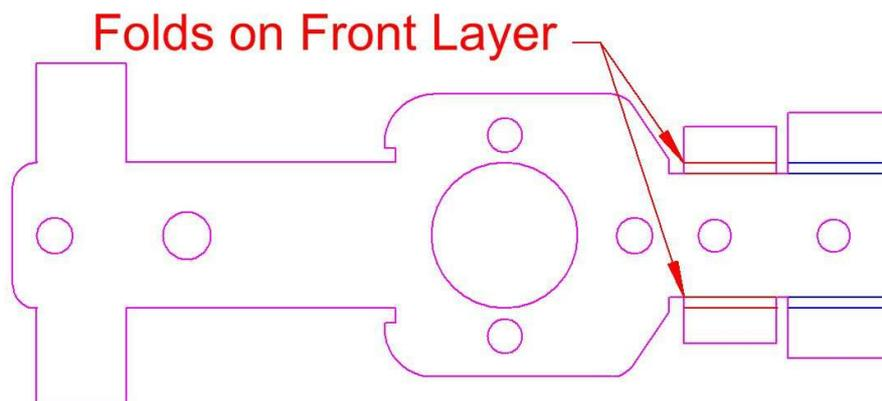
Next, the section forward, or on the left of X in the following picture needs to be bent upwards to stand at 90° to the section on the right. Therefore we need to create a fold across the part as shown at A. Because the fold is upwards, and the fold always closes the fold gap, it must be in red.
