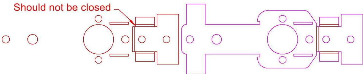
In drawing the outline of the part, we have closed the ends of the fold lines. This creates a number of intersecting lines that all end in a 'T' intersection. This T intersection will cause the Fill command to fail when the etching company tries to fill it later on. The reason is that Fill only recognises complete closed polygons, and does not like it when those polygons are connected to each other, as they are here.
