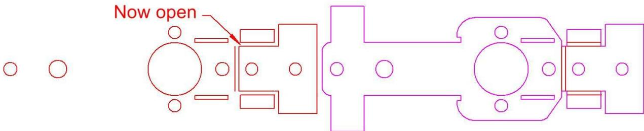
The ends can be opened by either removing the lines at the ends or by using the 'stretch' command to reposition the ends of the lines to their correct place. Another possibility is to use the 'trim' command to cut the ends out of the fold lines. Whatever works for you.
