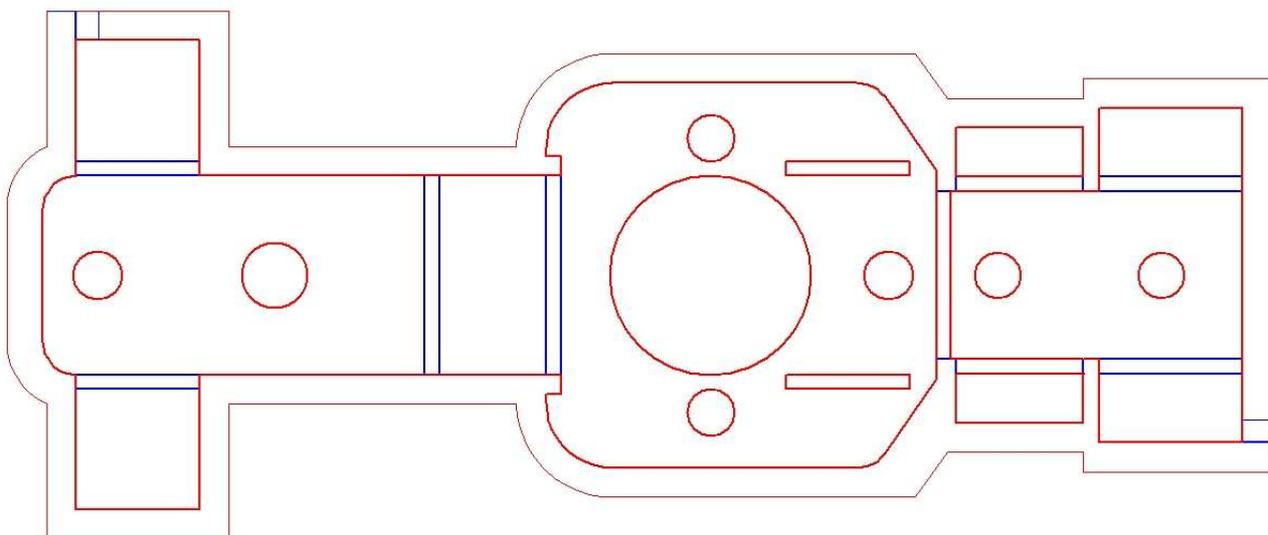
As a final test, before the completed component is inserted into the larger sheet of the fret, we should now fill each layer to make sure that all lines are joined properly. Switch off the front layer and apply fill to the rear layer, then switch the rear off, the front on and apply fill to the front layer.
