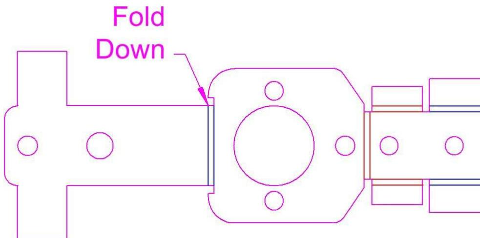
A further fold is required 3.25mm away from the last fold. The dimension 3.25mm sets the gap between the two cheeks of the gearbox where the gears and bearings will fit. This further fold is also downwards:
