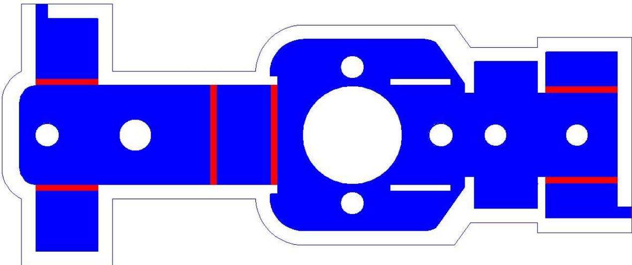
This does not look anything like the drawing you expect to see, so what has gone wrong? The fact that the main component itself seems to fill OK is an important clue. The problem is in the drawing of the moat, there is a small opening in the moat that allows the fill to 'leak' out. In this particular case, there is a tiny break between one of the circle segments and the connected straight line.
