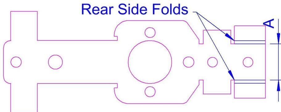
We need the dimension A to remain the same, as it is to locate the gearbox on the top of a brass channel, so the folds must be outside this width. The fold lines have been drawn in in blue on the rear layer.
