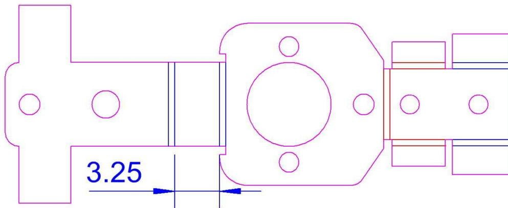
The final set of folds are the two tabs at F in the 3D picture. These tabs hold the front section of the gearbox a precise distance apart to allow the gears to sit in between.
