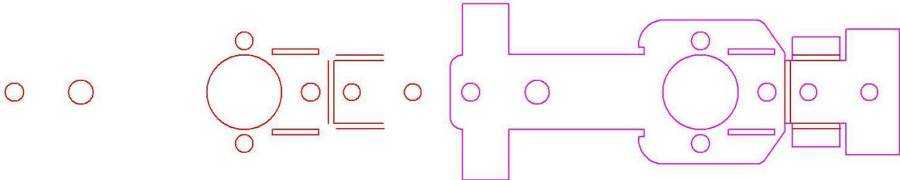
We can begin by drawing in the outline of the gearbox on the front layer, at the right hand end. This can simply be drawn over the top of the construction layer, using it as a guide. The left hand side would then look something like this:
