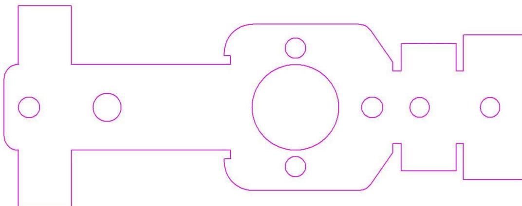
So far, the design has been drawn in purple on the 'construction' layer. This layer can be used to rough out the design before it needs to be drawn on the two etch layers. All that has been done at this stage is to accurately draw the gearbox to its correct size, as we imagine it would be folded out flat. All dimensions are so far correct and all holes in the right position. Looking again at the 3D view:
