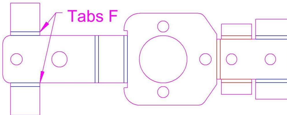
This completes the drawing of the folds in the gearbox. In order to positively locate the two tabs F in the drawing above, the best method is to create two slots for them to fit into. They can then be soldered into the slots to form a rigid cage for the gears.
