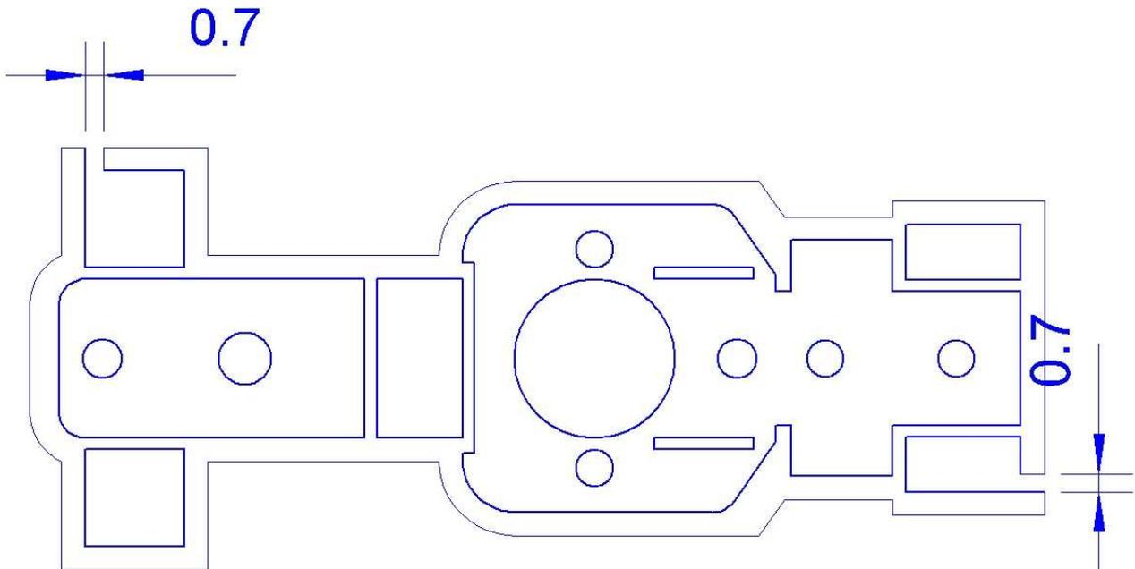
The tabs are not created on the top or red layer, as it is best if they are also half-etched, this makes them easier to cut. The resultant drawing should now look like this with both layers showing:
