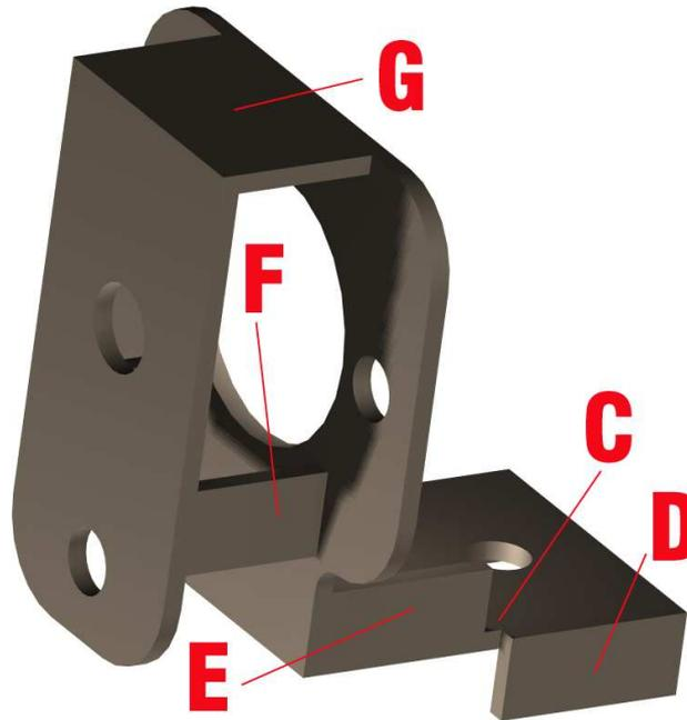
The locating tabs, shown as D above, need to be bent downwards as per our view. This means that a fold line needs to be drawn on the 'rear' or blue side of the drawing, bearing in mind our general rule of 'All folds are inwards'. As the material thickness is 0.45mm, we create two fold lines at the fold point, 0.45mm apart, as per the following drawing:
