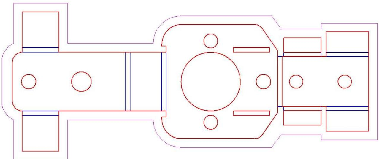
Having drawn the moat, duplicate it then assign one copy to the front layer and the other to the rear layer. Place the copies over each other in perfect registration. Switch off the red or front layer, leaving only the blue or rear layer.
