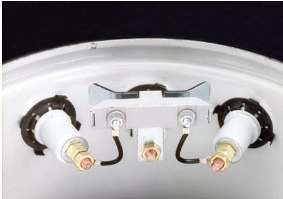
The spark gap mounted internally on the LV neutral bushing with the electrodes connected to the X1 and X3 bushings.
